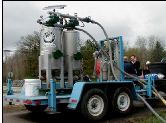
Sand Media Particulate Filter
