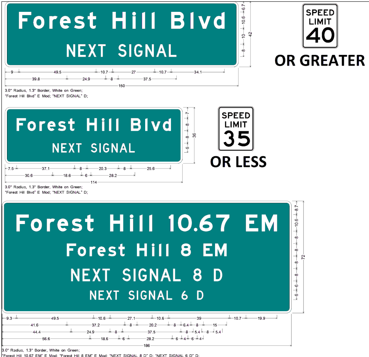
Figure 18 – 1 Examples of Advance Street Name Signs
