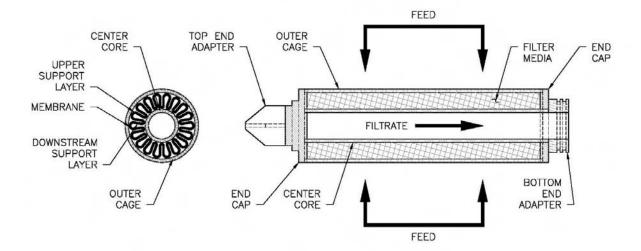
Figure 2.7 Membrane Cartridge Filter
