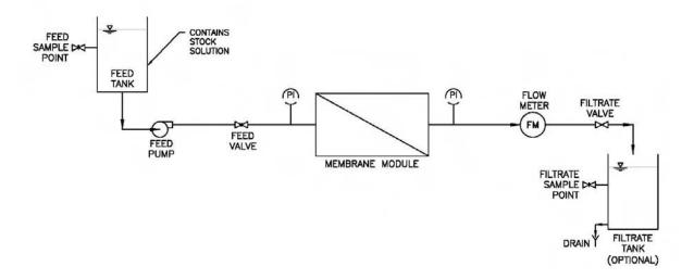
Figure 3.3 illustrates an apparatus similar to that shown in Figure 3.2, but designed for continuous in-line seeding and grab sampling rather than batch seeding and composite sampling. With this apparatus the challenge particulate is introduced from a stock solution reservoir and mixed prior to the feed sampling point. The use of grab sampling allows the collection of multiple feed and filtrate samples from a single test run.
