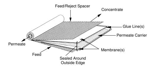
Spiral-wound membranes for drinking water treatment are commercially available in a variety of sizes. Modules that are either 4 or 8 inches in diameter and either 40 or 60 inches long are most common, although other sizes may be used. Some bench- and pilot-scale applications utilize modules that are 2.5 inches in diameter, while modules up to 16 inches in diameter or more may be used in full-scale facilities.
