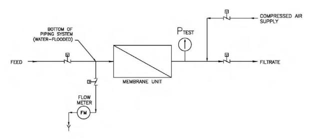
Figure 4.4 Schematic Illustrating a Water Displacement Test
