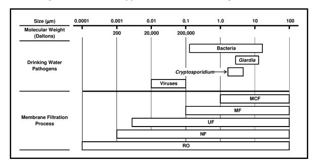
Figure 2.1 Filtration Application Guide for Pathogen Removal
