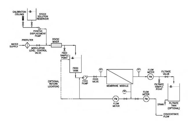
Figure 3.4 Schematic of a Typical Pressure-Driven System in Suspension Mode with Continuous Seeding and Grab Sampling
