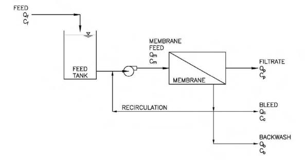
As with a CSTR without backwashing, the VCF for a CSTR with backwashing increases over time according to the first order exponential function given in Equation 2.35. However, in a CSTR with backwashing, the concentration of suspended solids on the feed side of the membrane is periodically reduced. Because filtrate is typically used in the backwash process, the backwash water introduces a negligible amount of particulate matter into the system; thus, it is
