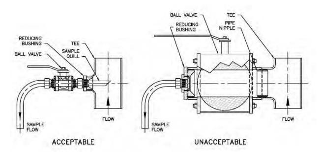
Figure 3.7 Schematic of Acceptable and Unacceptable Sampling Ports
