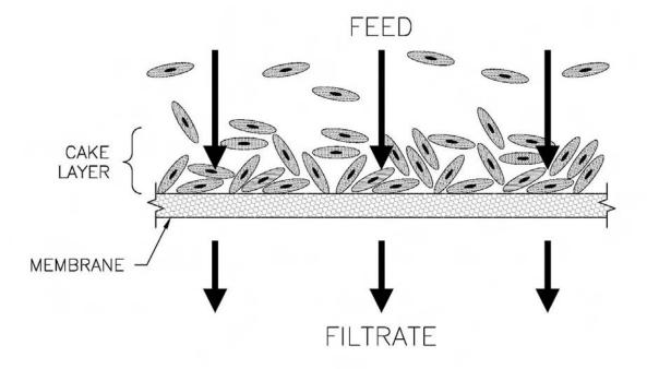
In a deposition mode hydraulic configuration, the concentration of suspended material on the feed side of the membrane  $(C_m)$  is assumed to be equivalent to the concentration of suspended material in the feed stream  $(C_f)$ , independent of time or position in the membrane system, as the suspended contaminants are removed from the process stream and deposited in the accumulated cake layer. Therefore, all systems operating in deposition mode have a VCF equal
