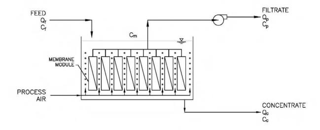
The VCF for a CSTR without backwashing increases as a function of filtration cycle time and can be defined in terms of the number of volumetric turnover times (i.e.,  $t/\tau$ ) and the recovery, as shown in Equation 2.35:
