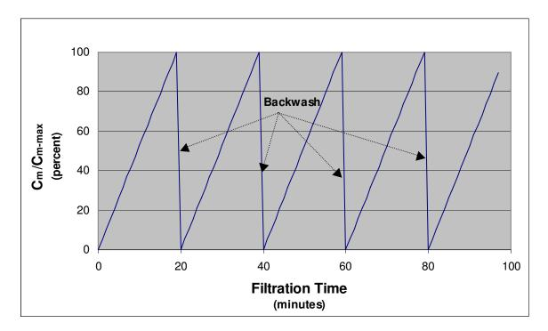
Since the VCF increases linearly from zero to  $VCF_{max}$  over the course of a filtration cycle in a crossflow system, the average VCF is simply one half of the maximum value, as shown in Equation 2.31:
