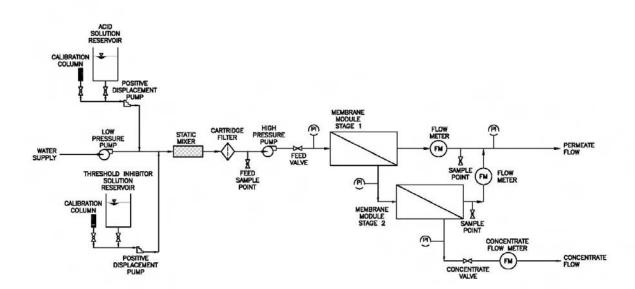
Figure 2.12 Schematic of a Typical Spiral-Wound (NF/RO) System
