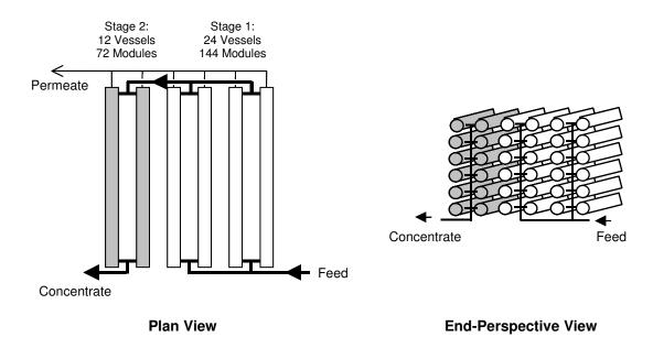
Figure 2.11 Typical 2:1 (Relative) Array of Pressure Vessels
