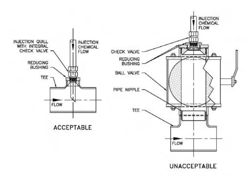
Figure 3.1 Schematic of Acceptable and Unacceptable Injection Ports
