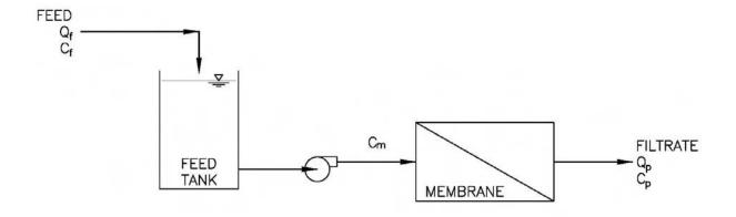
Figure 2.14 Conceptual Illustration of Deposition Mode Operation
