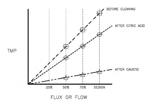
Figure 6.1 Sample Chemical Cleaning Test Profile
