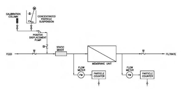
Figure 4.5 Schematic Illustrating a Particulate Marker Test
