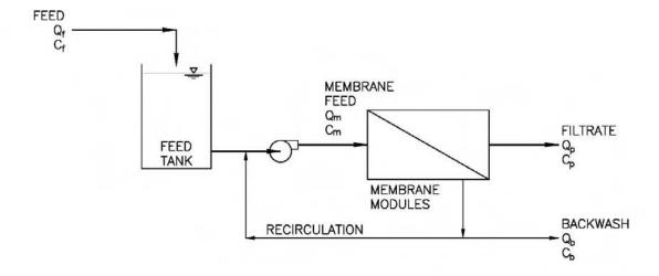
In crossflow systems, the concentration of suspended solids on the feed side of the membrane ( $C_m$  in Figure 2.17) increases linearly over the filtration cycle. The rate at which the concentration increases is a function of the feed flow ( $Q_f$  in Figure 2.17) and volume of the recirculation loop ( $V_r$ ). As shown in Figure 2.17, this volume would include the volume on the
