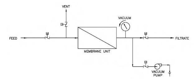
Figure 4.2 Schematic Illustrating a Vacuum Decay Test
