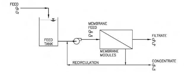
Figure 2.22 Schematic of a Typical Vacuum-Driven CSTR Without Backwashing
