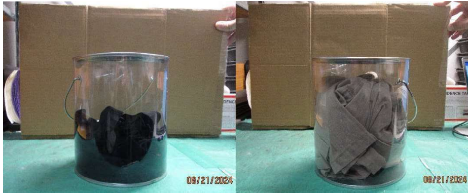
Image 2. Example of a proper amount of sample inside the container (Left) and an improper amount of sample inside of the container (Right).
