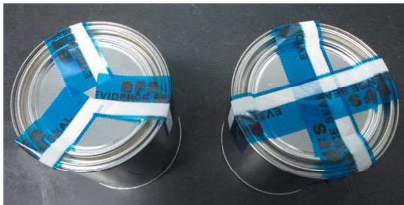
Image 1. Examples of proper tape seals.
