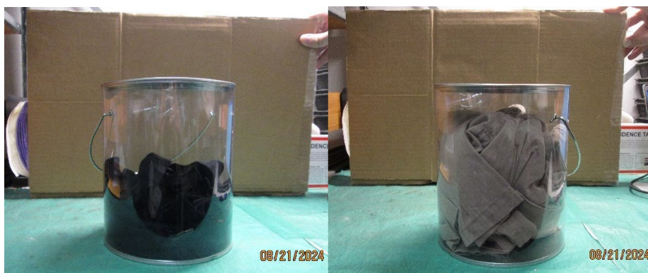
Image 2. Example of a proper amount of sample inside the container (Left) and an improper amount of sample inside of the container (Right).
