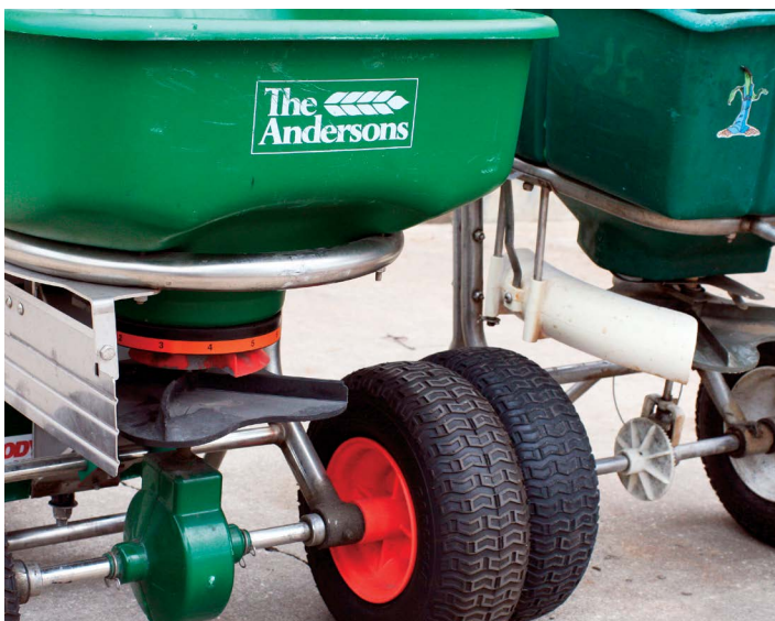
Figure 21. Spreaders with deflector shields.
