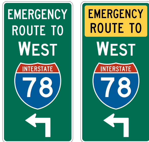
Examples of guide signs for rerouting
