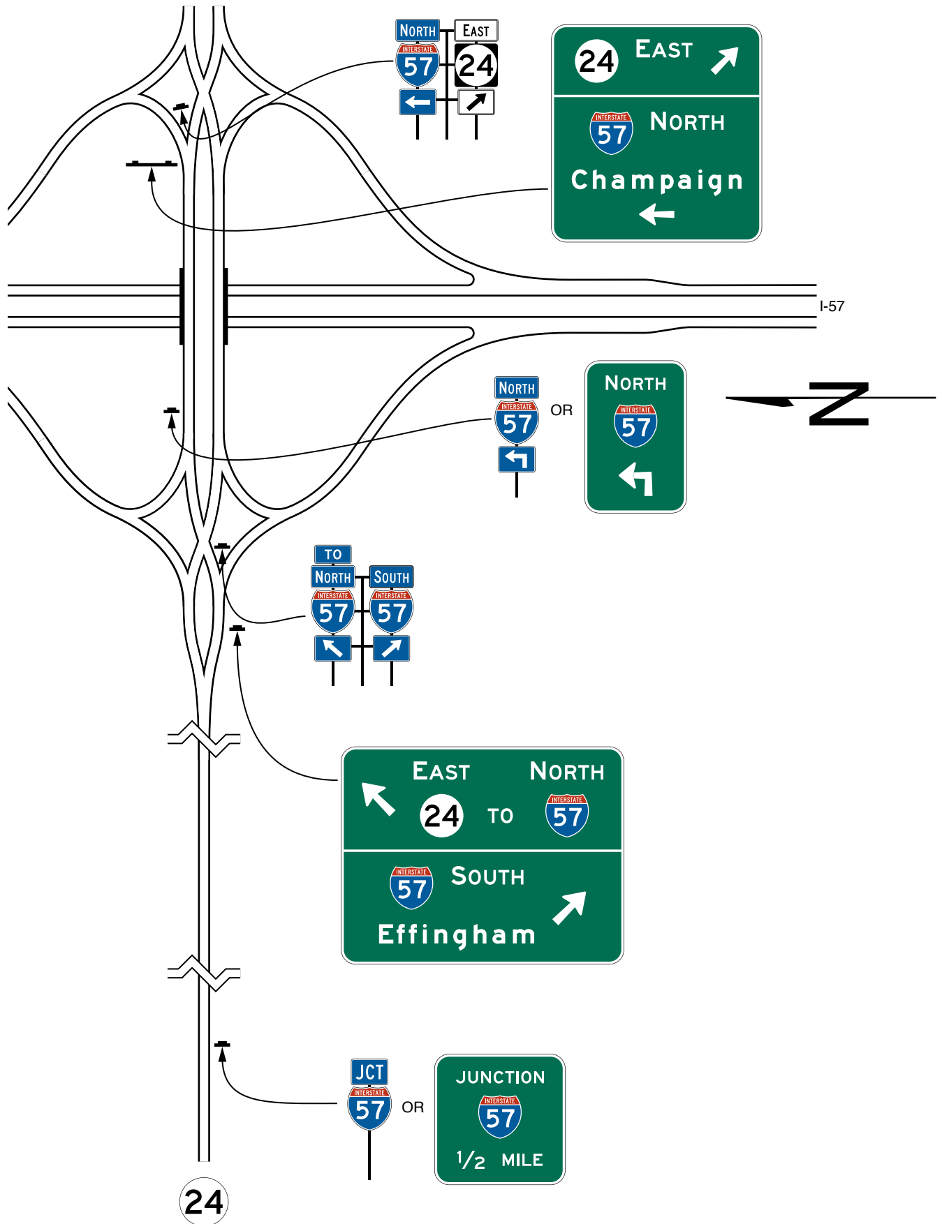
Figure 2D-21. Example of Transposed Alignment Crossroad Guide Signing at a Diamond Interchange
