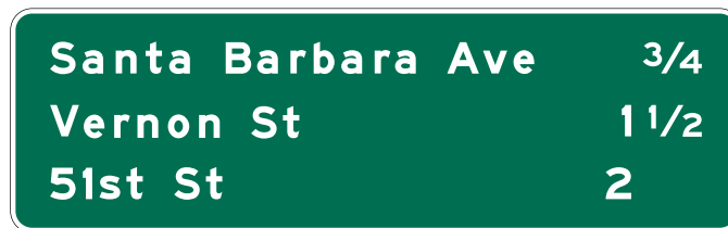
Figure 2E-10. Example of an Interchange Sequence Sign
