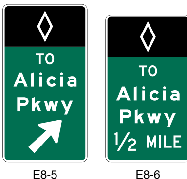
Figure 2G-12. Examples of Barrier-Mounted Guide Signs for an Intermediate Egress from Preferential Lanes
