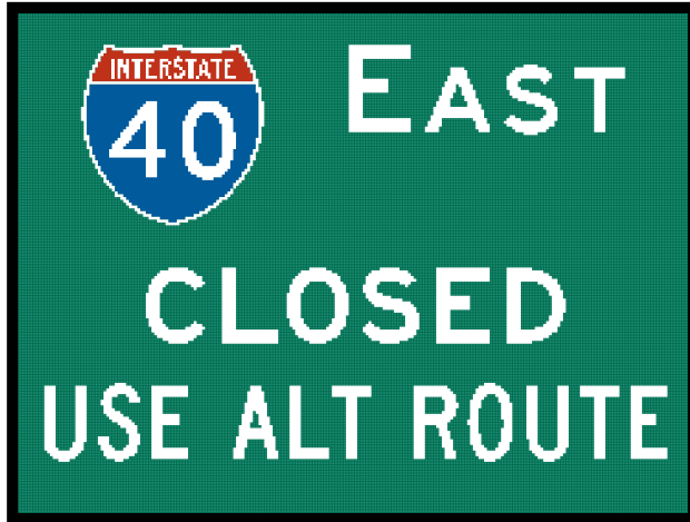
Figure 2L-1. Example of CMS Capability to Display Sign Legends Based on Pixel Pitch
