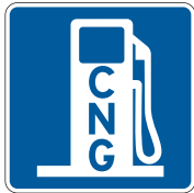
D9-11a Alternative Fuel- Compressed Natural Gas
