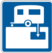
D9-12 RV Sanitary Station
