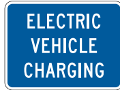
D9-11bP Electric Vehicle Charging
