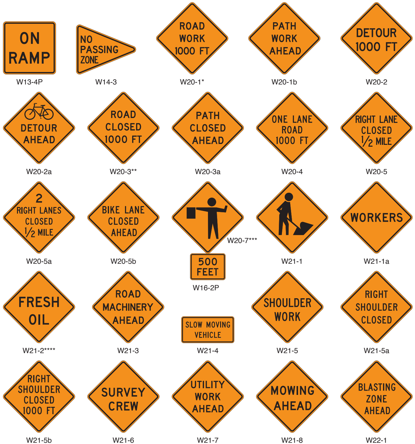
Figure 6H-1. Warning Signs and Plaques in Temporary Traffic Control Zones (Sheet 3 of 4)
