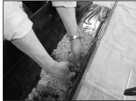
Figure 3-19. Loosening the Clumps of Bedding Material.
