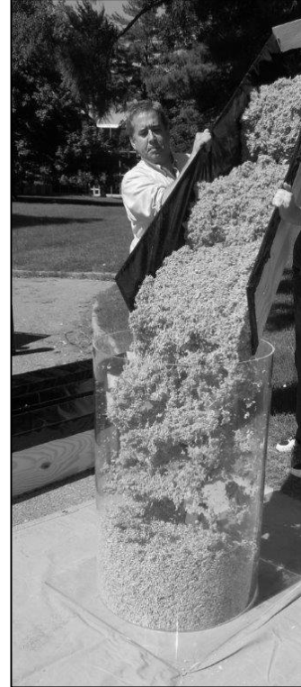
Figure 3-24. Filling a Test Measure at an Angle to use the Larger Opening.
