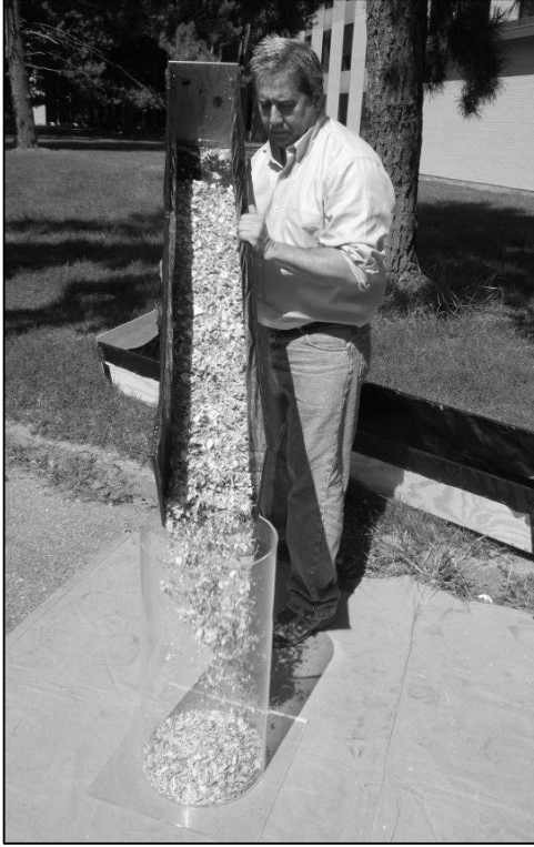
Figure 3-23. Filling a 44 L Test Measure.
