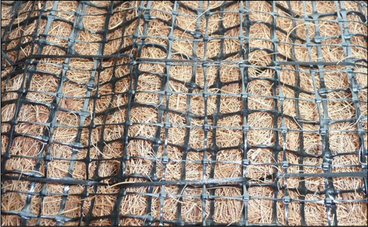
Figure 2.6 Example of Geogrid Mat (source: RH Moore)
