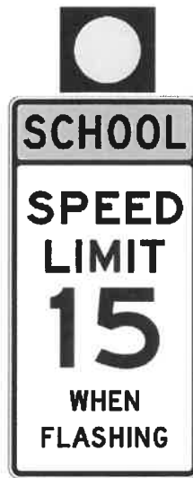
15 MPH School Zone Roadside Flashing Beacon Assembly (MUTCD S5-1)
