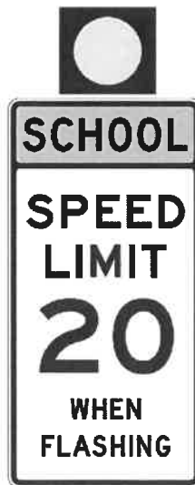
20 MPH School Zone Roadside Flashing Beacon Assembly (MUTCD S5-1)
