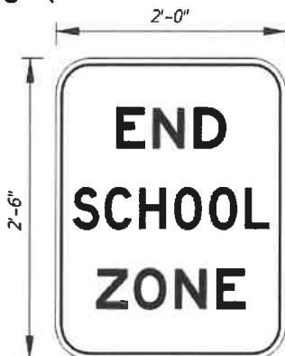
Figure 15-9A End School Zone Sign (Ground-Mounted Option – FTP 34-06)
