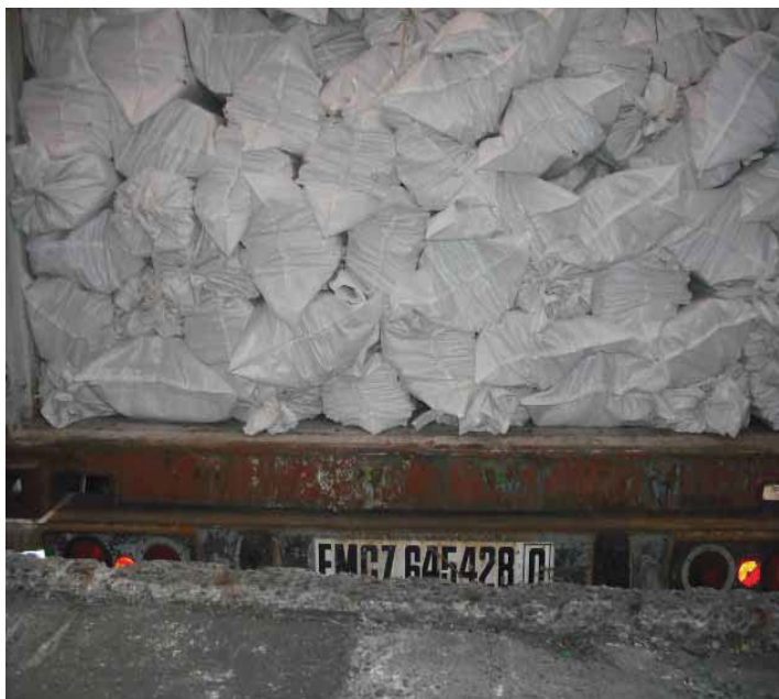
Figure 5-5-1 Example of Inadequate Spacing Under Bamboo Bundles
