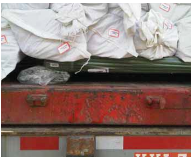
Figure 5-5-2 Example of Inadequate Spacing Under Bamboo Bundles
