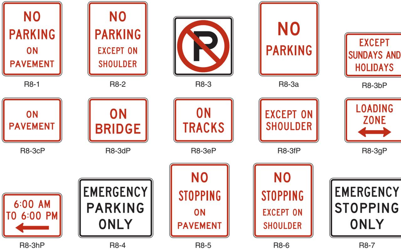
03 Where parking is prohibited at all times or at specific times, the basic design for parking signs shall have a red legend and border on a white background (Parking Prohibition signs), except that the R8-4 and R8-7 signs and the alternate design for the R7-201aP plaque shall have a black legend and border on a white background, and the R8-3 sign shall have a black legend and border and a red circle and slash on a white background.
