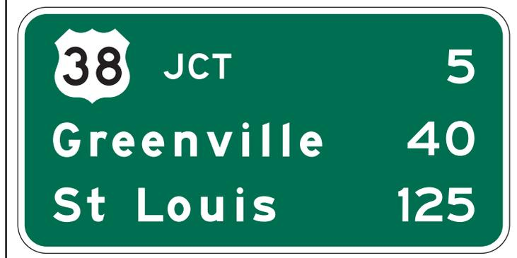
**Figure 2E-30. Example of Using an Interchange Sequence Sign for Closely-Spaced Interchanges**
