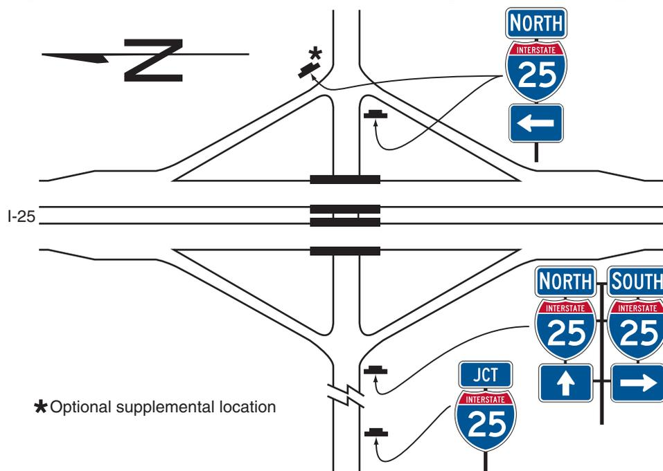
Figure 2D-14. Examples of Multi-Lane Crossroad Signing for a Partial Cloverleaf Interchange
