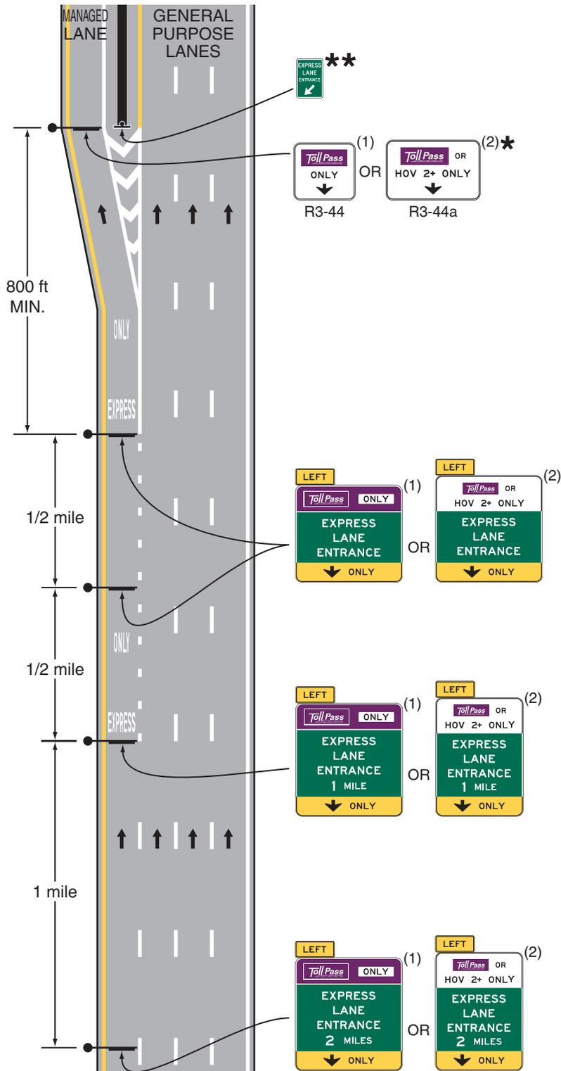
**Figure 2G-23. Example of Signing for an Intermediate Entry to a Barrier- or Buffer-Separated Priced Managed Lane**
