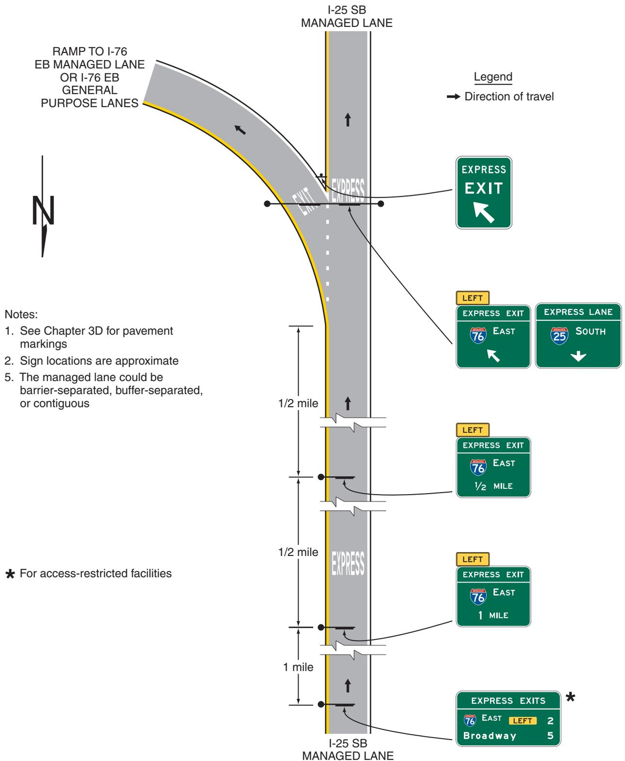
**Figure 2G-29. Examples of Guide Signs for Separate Entrance Ramps to General-Purpose and Priced Managed Lanes from the Same Crossroad**
