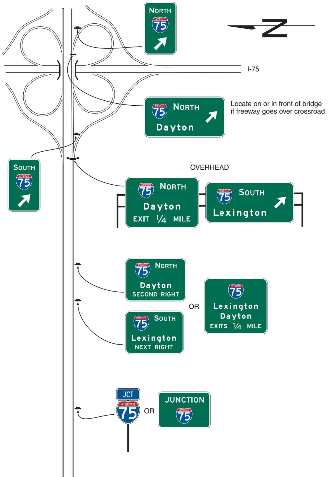
**Figure 2D-16. Example of Crossroad Signing for an Entrance Ramp with a Nearby Frontage Road**
