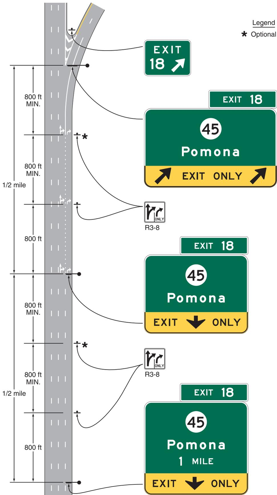
**Figure 2E-12. Example of Signing for a Two-Lane Intermediate or Minor Interchange Exit with Option and Auxiliary Lanes**
