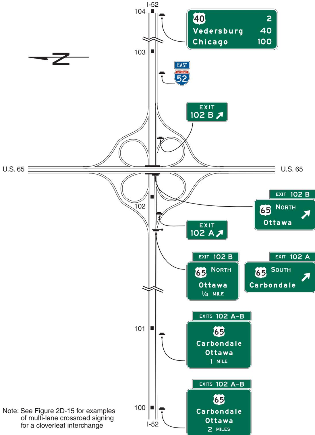
Note: See Figure 2D-15 for examples of multi-lane crossroad signing for a cloverleaf interchange
