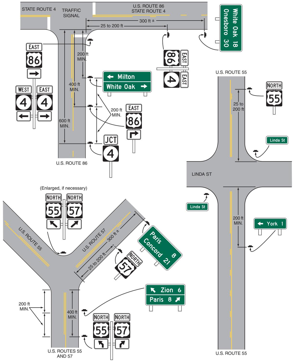
Note: The spacings shown on this figure are for rural intersections. See Sections 2D.29, 2D.30, 2D.32, 2D.34, 2D.40, and 2D.42 for low-speed and/or urban conditions.
